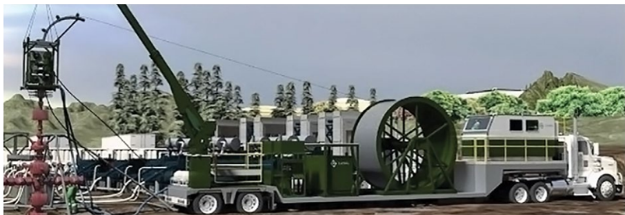
Ziebel's fiber-optic sensing tool is run downhole to capture DTS and DAS data for production logging and well calibration.
