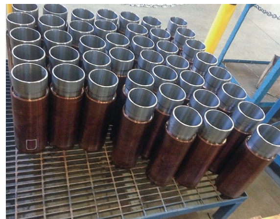
Since 2006, ConocoPhillips has continued to progress the use of flow control devices in its SAGD operations in Canada, using field trials and lab tests. Wells with FCDs show a marked reduction in circulation time and a substantial uplift in production.
