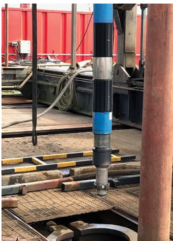
Foro Energy's laser technology can cut through conductor pipe, production tubing and cement.
